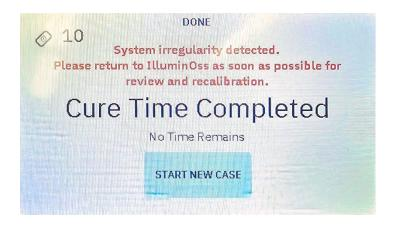
NOTE: Any minor system faults that occur during the curing cycle shall automatically generate the warning that the system operated outside of its established parameters and that a second curing cycle is required.
