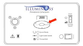
CAUTION: FAILURE TO USE THE PROPER VARIABLE TIMER KEY CAN RESULT IN INADEQUATE CURING OF THE IL-LUMINOSS MONOMER. ENSURE YOU ARE USING THE CORRECT TIMER KEY CORRESPONDING TO THE IMPLANT SELECTED FOR SURGERY.
